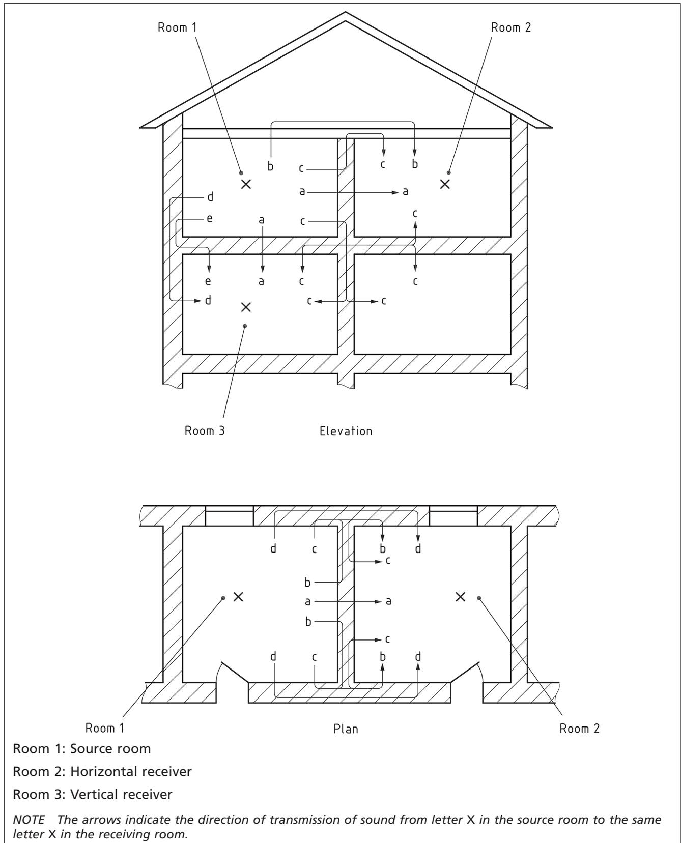
Figure E.2 Indirect sound leakage paths
