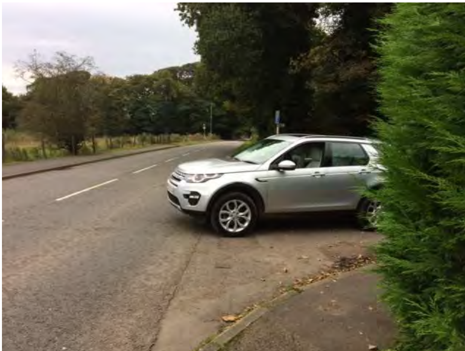
Vehicle position at junction for clear view to right. For clear view to left vehicle is required to be even further into the carriageway
