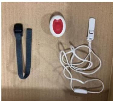
The neck cord has a plastic attachment attached to it. Push this through the back of the red/cream button so that it clicks into place and secures itself.
