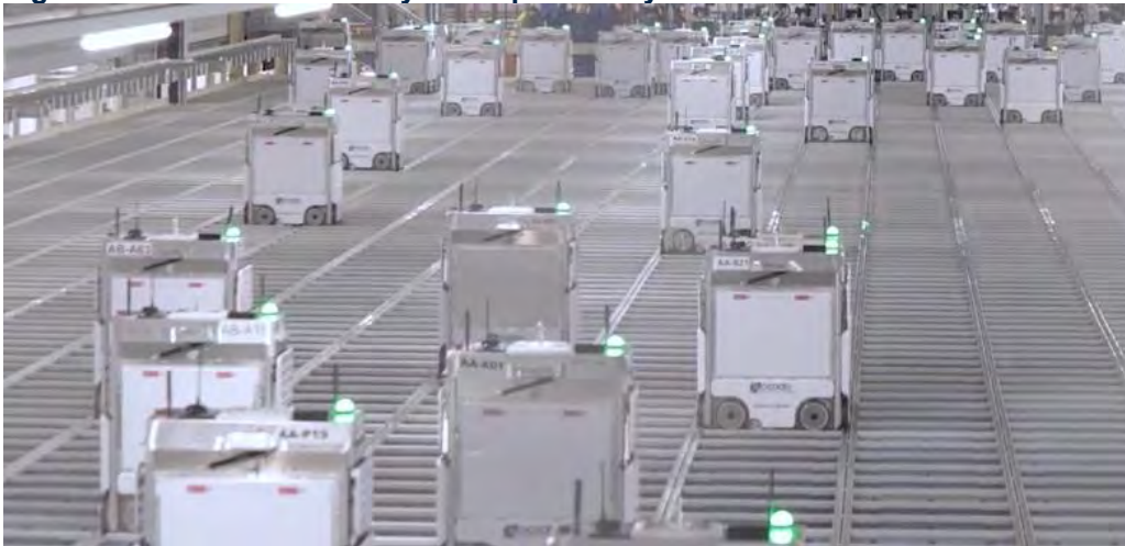
Figure 10.6 The automated system operated by the ‘Ocado Smart Platform’
